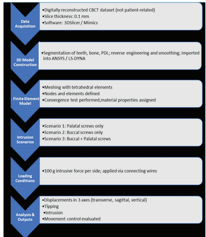
Figure 1. Flowchart summarizing the study design. The process included CBCT dataset reconstruction, 3D segmentation, finite-element meshing, simulation of three intrusion scenarios (palatal screws, buccal screws, and combined anchorage), application of a 100-g intrusive force per side, and evaluation of displacement, tipping, and intrusion patterns.
