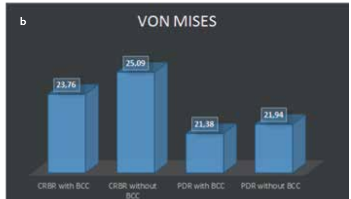
FIGURE 4. a, b. Stress values of restorative materials used as enamel replacement (a). Stress values of restorative materials used as core and substructure (b) CRBR: coronal-radicular build-up restoration; BCC: buccal cusp coverage; PDR: post-retained direct restoration.
