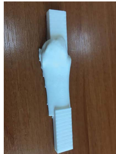
FIGURE 1. 3D printed distal tibia model with anatomical reduction on CT images of the patient.
