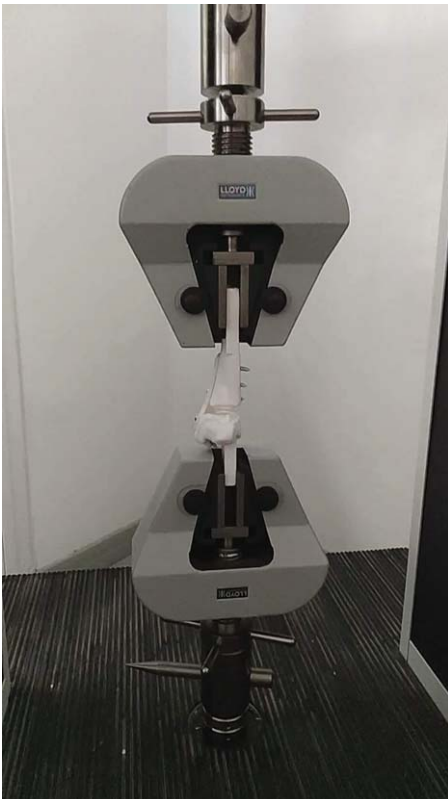
FIGURE 3. Tibia model with implanted plate on Lloyd-Ametek EZ-50 Material Testing Machine.
