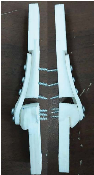
FIGURE 2. The implanted PLLA plate on the bone model with full contact. (a) Posterior view; (b) anterior view.
