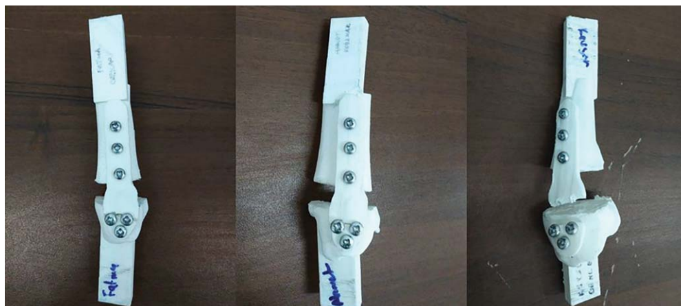
FIGURE 6. Samples showing the breakage zones of the 3D printed plates.
